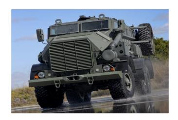
OFB has developed and supplied Mine Protected Vehicles (MPV) to Indian Army and Para-military forces, which has a capability to withstand blast of 14 Kg TNT under the wheels and 10 Kg TNT under the hull.
