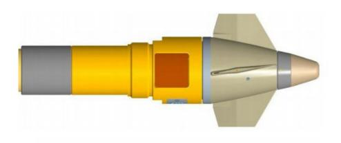
Fitment of PGK on existing ammunition improves accuracy (CEP- Circular Error Probability) of the Ammunition from 250 to 50 Mtrs. OFB has associated with DRDO from design stage to develop PGK for 155mm Ammunition.
